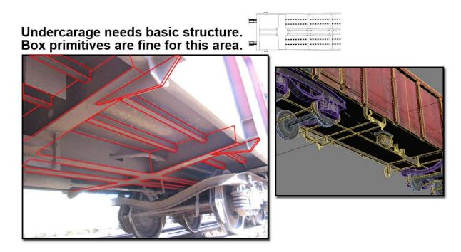
8. Details and proportions of car controls should be modeled to look appropriately dimensional when being viewed from any angle to the side of the car. Also, maintain a close relationship to the proportions seen in the reference materials.
